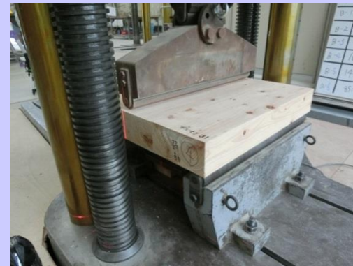
Panel shearing test
