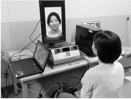
Figure 1. The experimental apparatus and setting. The laptop PC at the left processes stimulus displayed on the monitor located at the center. The eye-tracking detection unit is located in front of the monitor, and desktop PC at the right is control unit used for calibration.
