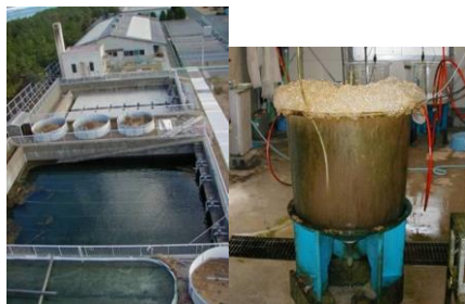
Fig.2 The size of culture tank was minimized to 1/100 in our high density culture system (right) from the classical culture system (left) to produce the same amount of rotifer
