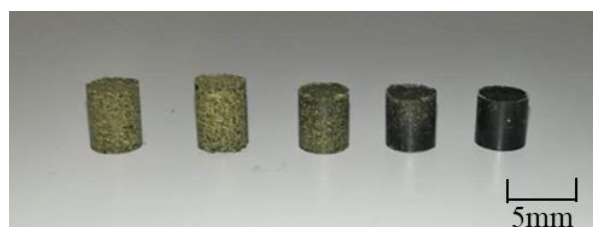
Fig. 5 Surface appearance of green tea biocoke for each molding pressure at molding temperature 383 K
