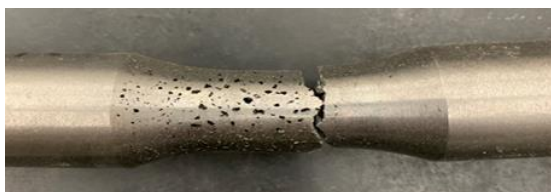
Fig. 2 Tensile test piece (Diameter of parallel part : 20 mm)
