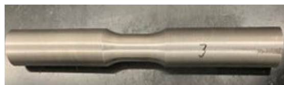
Fig.3 Tensile test piece (Diameter of parallel part : 20mm)
