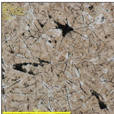
Fig. 4 Metallographic structure of cast iron
